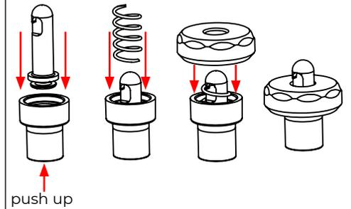
3. Hold assembly by placing thumb on bottom of seat cup and two fingers on either side of stem. Hook opening should be facing away from your hand.
