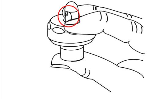
4. Hold handle in other hand. Make sure hook opening is facing front of handle as shown.
