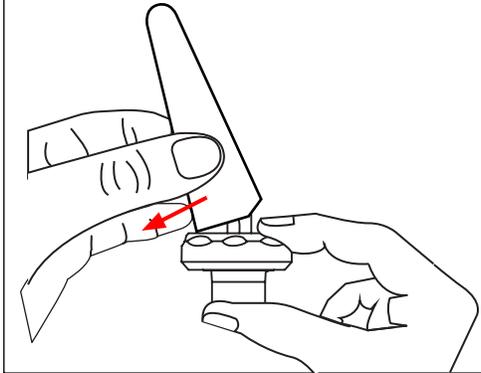
2. Place stem in seat cup. Push up on bottom of the seat cup until the stem pops into place. Place spring over stem. Place bonnet over stem.
