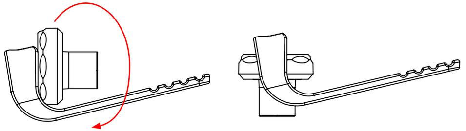
2. Place thumb on bottom of seat cup and two fingers on bonnet.
