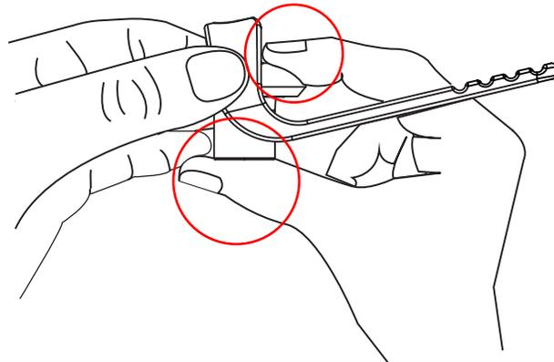
3. Pinch bonnet and seat cup together by pushing up with your thumb. Angle pieces out until the stem is unlatched from the notches. Be cautious to let go slowly as spring will release.
