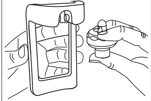
5. Align Hook opening with notches in the handle. Push up on seat cup so the stem rises.
