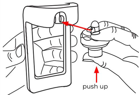
6. Push bonnet forward with thumb until hook opening latches onto the notches in the handle.
